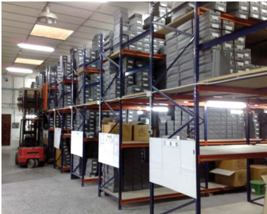
Products are warehoused on the basis of shoe model, without pallets
