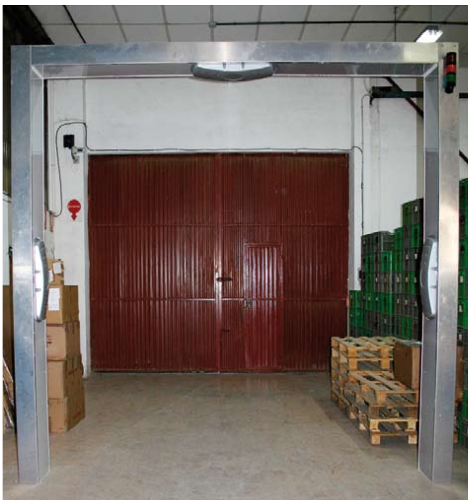
The portal automatically detects any incoming or outgoing movements
